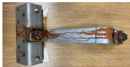
6. Sample of acid-resistant steel 1.4301 with an A2 stainless steel screw after a full cycle of 720 h.
