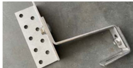
2. Before putting into the salt chamber a sample of acid-proof steel 1.4301 with an A2 stainless screw.
