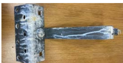
5. Photo of a magnelis sample with a hot-dip galvanized bolt after a full cycle of 720 h.
