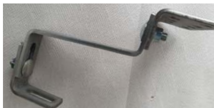
1. Photo before putting the magnelis sample with a hot-dip galvanized bolt in the salt chamber.
