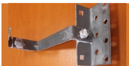
3. Photo of the magnelis sample with a hot-dip galvanized bolt after 320 h.
